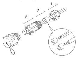
Fix the cable. This sign must be on top:
